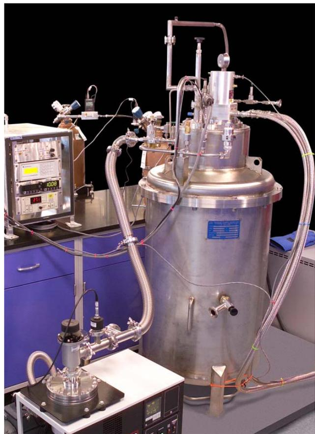
**FIGURE 1. A 150L liquid hydrogen densification and zero-boil-off storage system at FSEC.**
